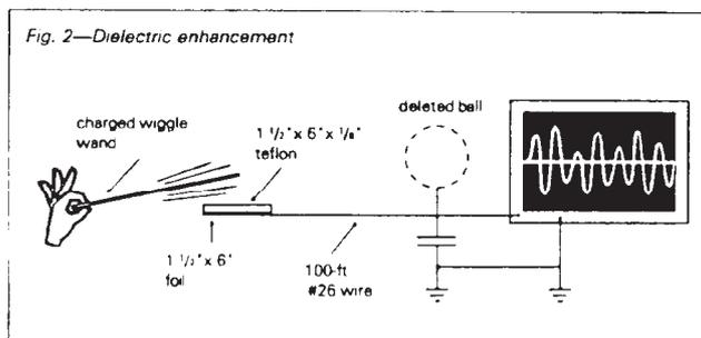
Experiment VI: If the ball antenna is replaced by a flat foil surface covered by a 1/8" layer of Teflon, (see Fig. 2) the static charge transmission signal is greatly enhanced. In fact, simply touching the Teflon surface and making slight movements, or touching the surface intermittently, transmits strong signals. We are talking two to three volts,
