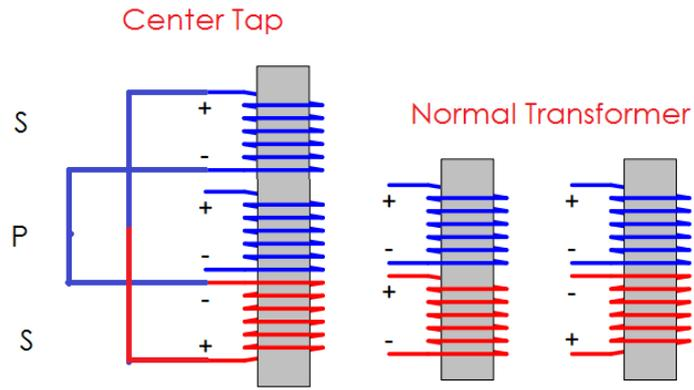
Depending on how the coils are wound, the polarity of the voltage on the secondary to the primary has either direction. I.e., we have the voltage on the secondary in phase (left image) or in opposite phase (right image) with the primary voltage.
