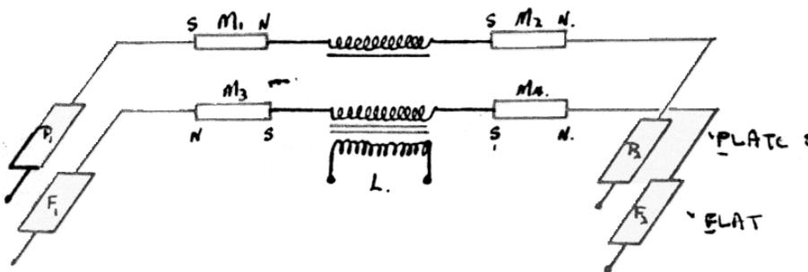
This device consists of an arrangement of magnets, flat coils, and copper plates, with a primary circuit energized by a small dry battery. The output from the secondary was used to light a bank of lamps and was claimed to be many times the original input, and to continue indefinitely. Details of this circuit, and a theory as to its mode of operation were given (summarized in Appendix I).
