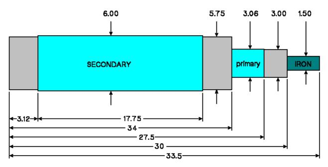
Now wire the two coil assemblies as shown below. Try to start the device by swiping a powerful magnet along the coils or the core. Try different resistor values. Try shorting the outputs. Try putting light bulbs across each of the two outputs. Test with meter.
