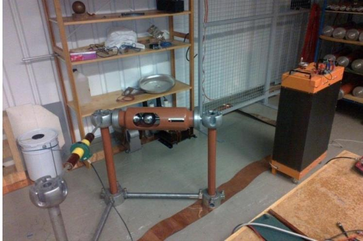
**Fig. 33: Complete setup of the experiment to find out indirect parameters of arc (Photo: Tatu Nieminen)**
