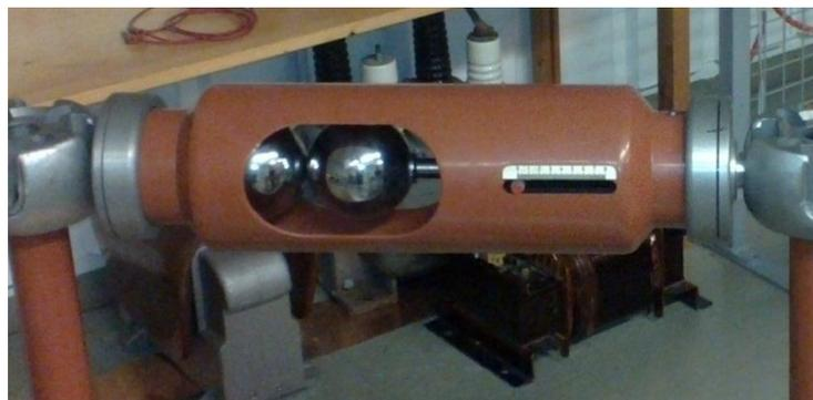
**Fig. 32: The electrodes with about 0.11mm gap used for the experiment (Photo: Tatu Nieminen)**
