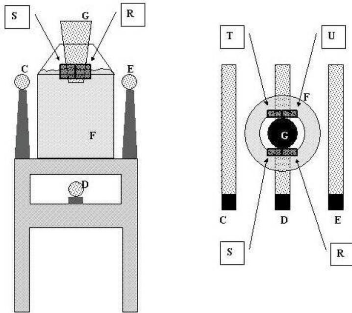
**Fig. 7:** Layout of the experimental setup of the second investigation showing the position of the boron screened CR39 plates with respect to the rest of the equipment.
