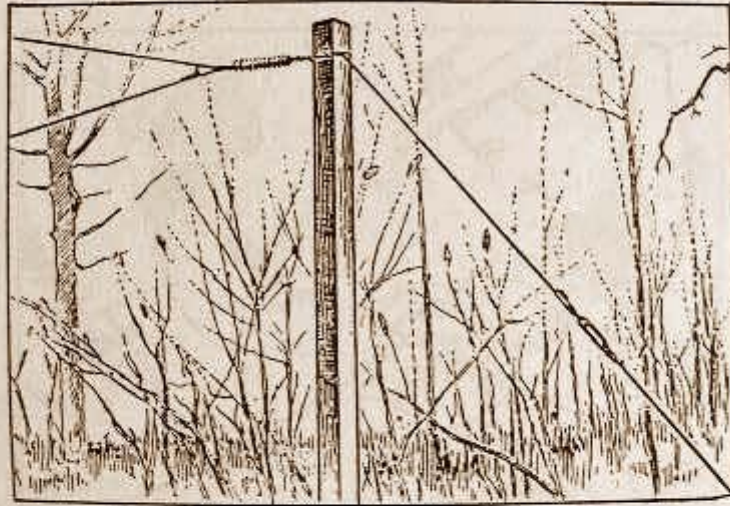
Fig. 115.—Method of holding overhead wires to posts
