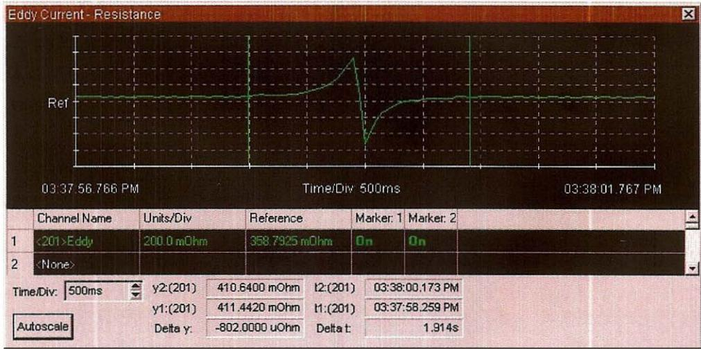
The resistance at the maximum is 880.21mΩ and at minimum is -162.63mΩ with a reference resistance of 358.79mΩ. Therefore, at first we see that the change in resistance is exactly 521.42mΩ both above and below the reference resistance. The interval from the
