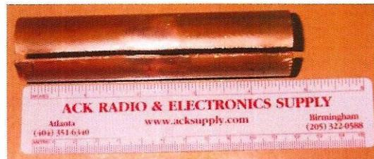
Figure 3. Copper tube with slit along length.
