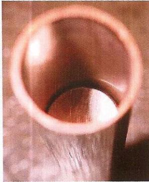
In an effort to test this theory, a NIB magnet drops down a copper tube. The magnet is 1" in diameter and nearly 1/4" thick.
