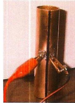
We attached an HP 34970A data acquisition switch with a built in digital multimeter to test for resistance. Two terminals were soldered mid-length, one on each side of the slit as in the image to the right. We cleaned the terminals to assure a good contact.
