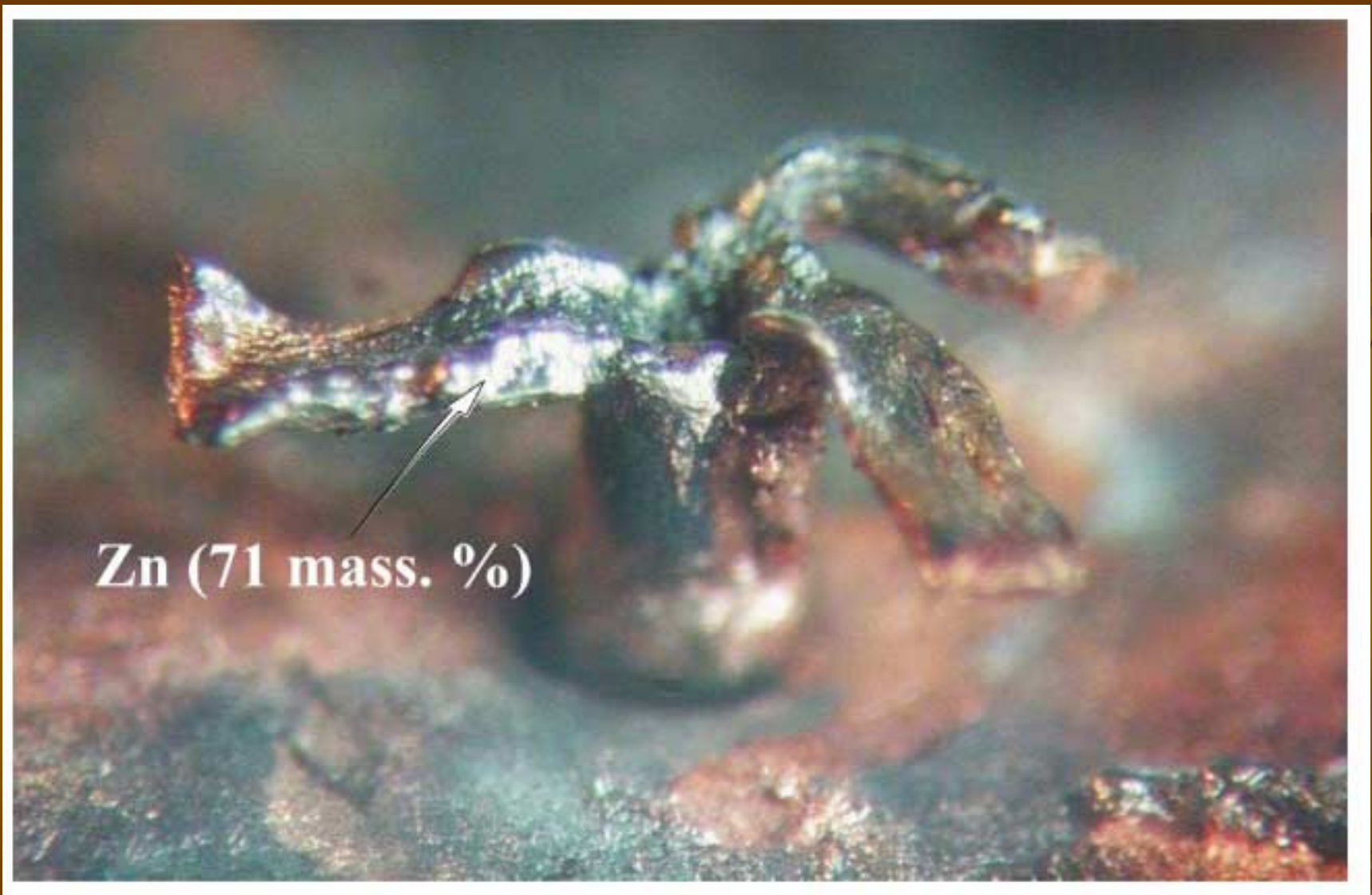
Copper target after the experiment, with traces of solidified silver-and-white “lava” on its “petals”, which had flowed out of the target center.
