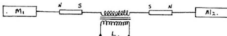
The basic element is that of an open secondary circuit, capacity loaded, inductively coupled to a primary circuit. The novel feature is that the capacities are connected to the secondary core through permanent magnets, as shown.
